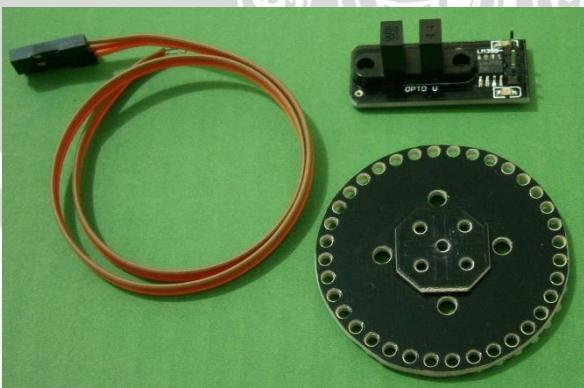
Gambar 2.12 Rotary Encoder
