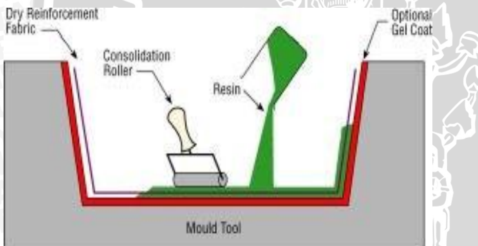
Gambar 2.5 Metode Hand Lay Up Sumber : (Faisal,2011)
