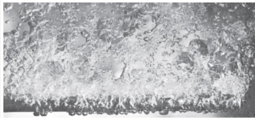
Gambar 2.9 Nucleate boiling
