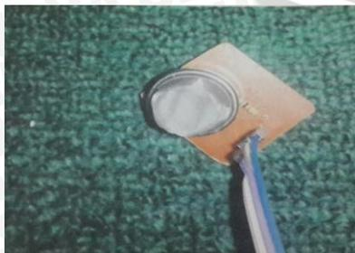
Gambar 3.11 Sensor gas  $H_2$
