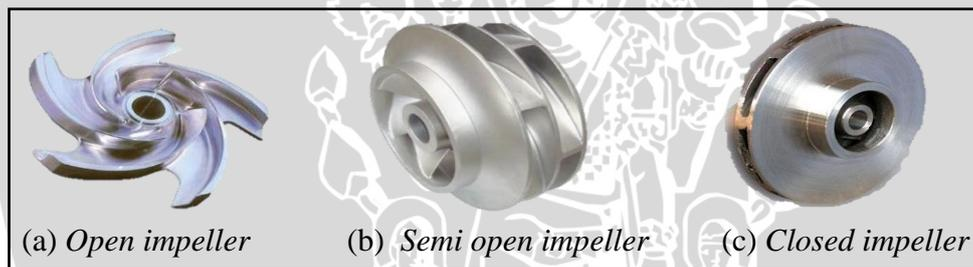
**Gambar 2.34** Macam – macam *impeller*
