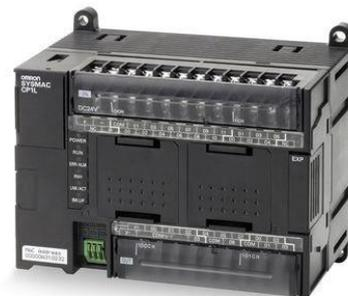
Gambar 3. PLC Omron CP1L-L20Dxx
