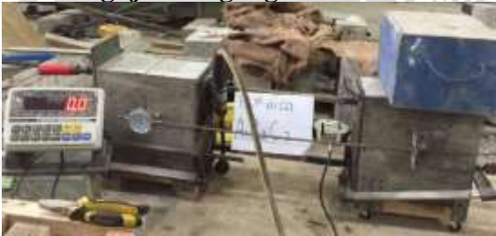
Gambar 4.2 Setting pengujian pull-out
