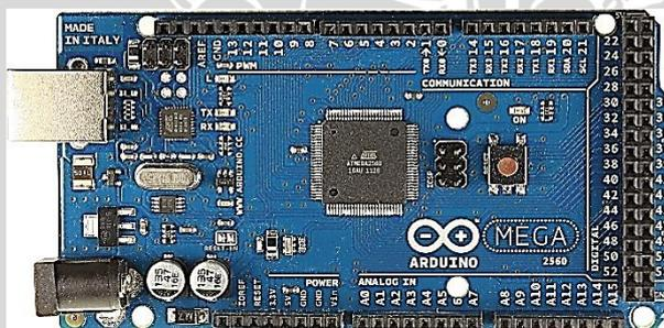
Gambar 2.1 Arduino Mega 2560
