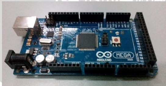
Gambar 3.16 *Arduino Mega 2560*
