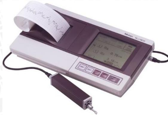
Gambar 3.3 *Surface Roughness Tester* Mitutoyo SJ 301.
