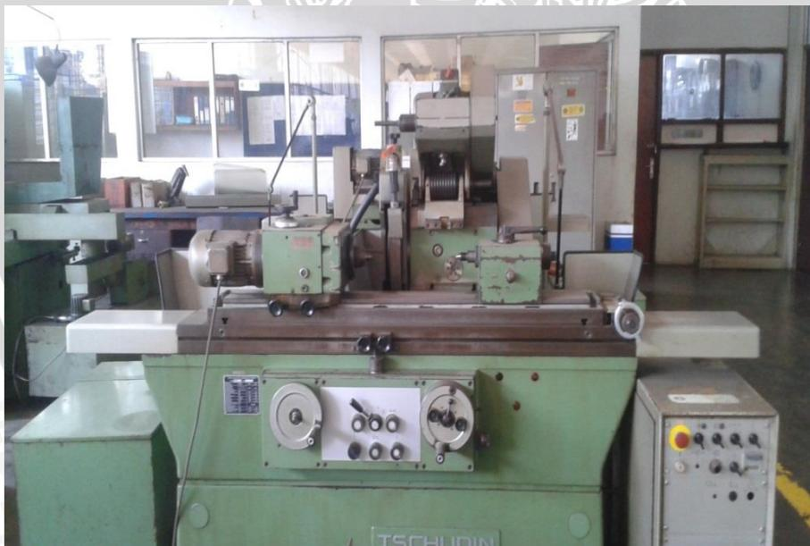
Gambar 3.1 Mesin Gerinda Silinder Tschudin HTG 610 82 200
