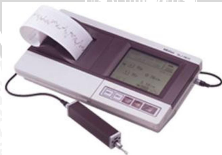
Gambar 3.3 Surface Roughness Sumber: Lab. Metrologi Industri
