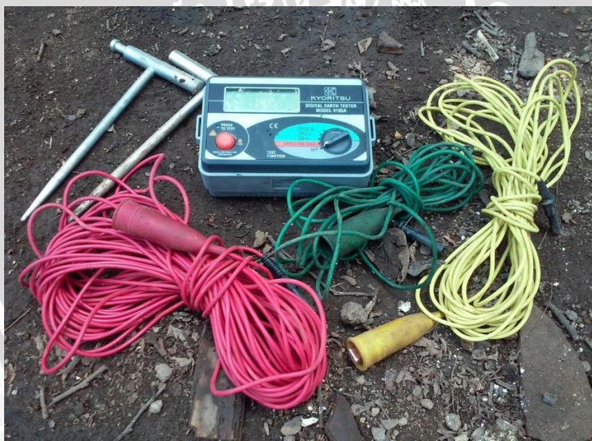
Gambar 4. Alat ukur digital earth resistance tester 4105 A
