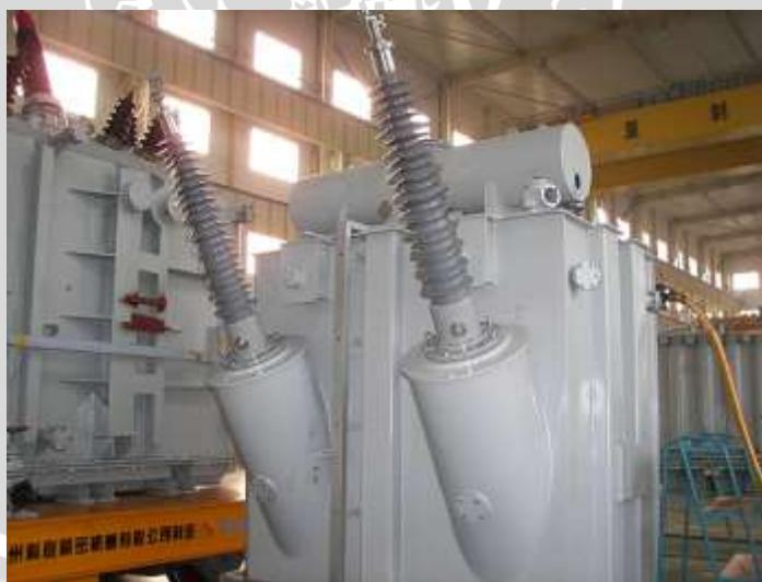
**Gambar 2. 4 Bushing Transformator**
