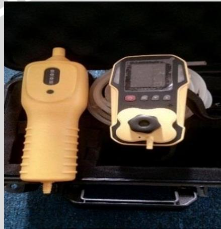
Gambar 3.1 Gas Analyzer (Biogas Detecting Alarm)
