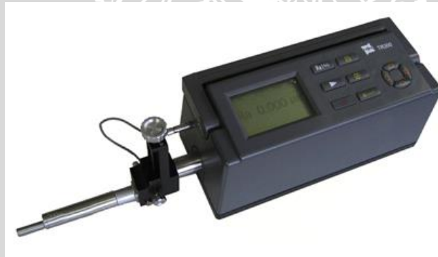
Gambar 3.2 Surface Roughness Test
