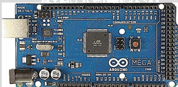
Gambar 2.1 Arduino Mega 2560
