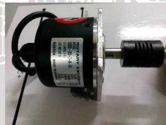
Gambar 4.5 Rotary encoder Autonics E50S8-360-3-N-24
