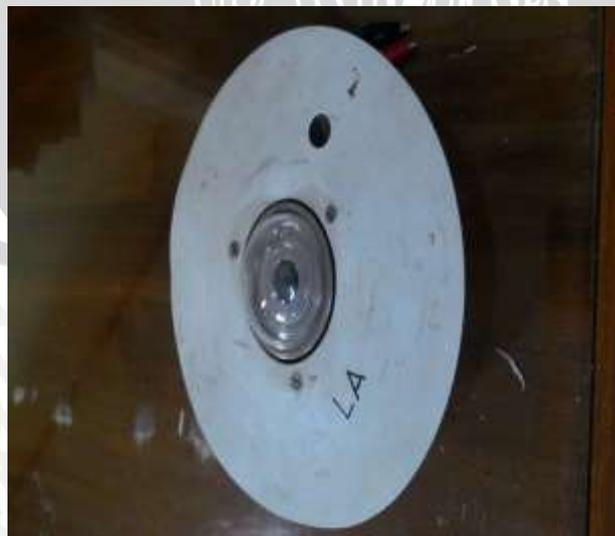
Gambar 3.6 Pyranometer
