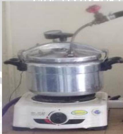
Gambar 3.2 *Boiler air*
