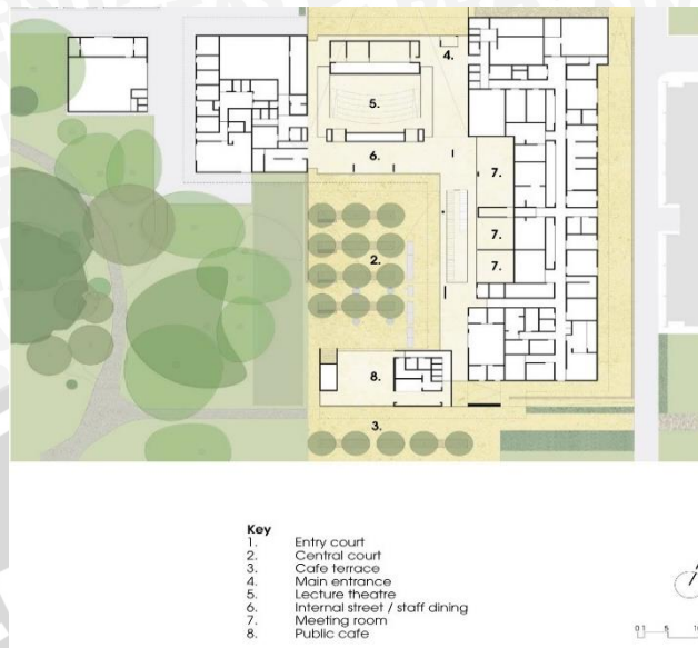
Gambar 2.31: Denah lantai 1 Sainsbury laboratory
