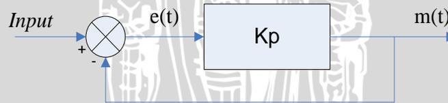
Gambar 2.6 Diagram Blok Kontroler Proporsional
