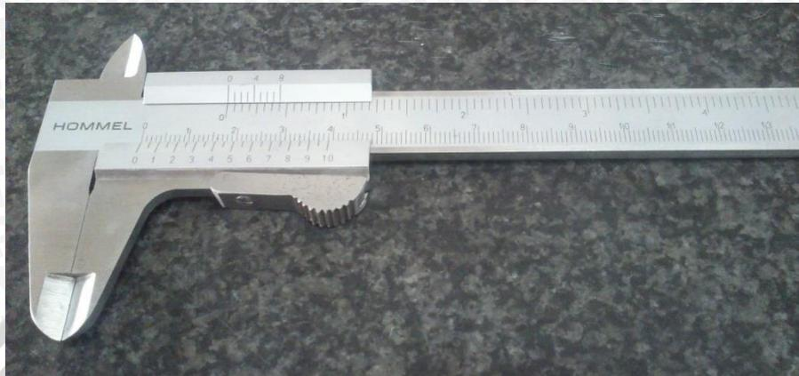
Gambar 3.2 *Vernier Caliper*
