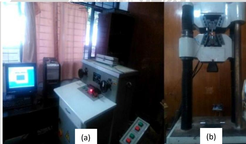
Gambar 3.5 Mesin Uji Tarik (a) *Display controller* (b) *Specimen holder*
