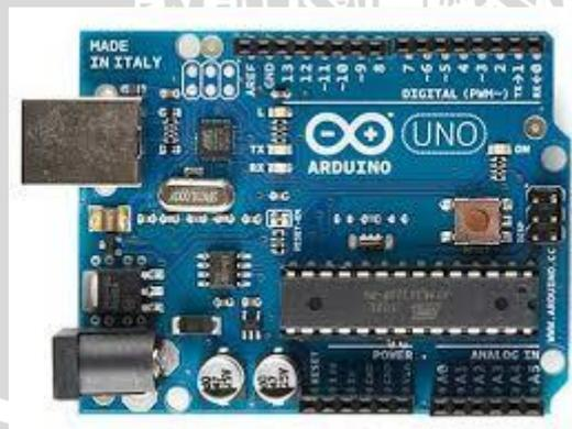
Gambar 4.1 Modul Arduino Uno
