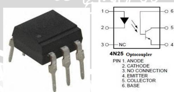
Gambar 2.13 Optocoupler 4N25 (Datasheet)
