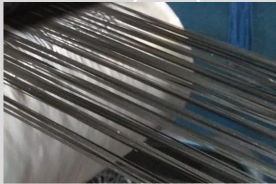
Gambar 1.5 Benang pipih hasil proses extrusion
