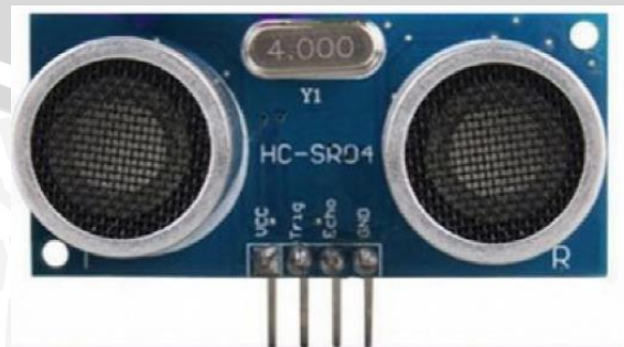
Gambar 2.4 Sensor Jarak HC-SR04
