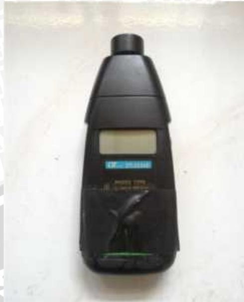
*Gambar 3.2 Digital Tachometer*
