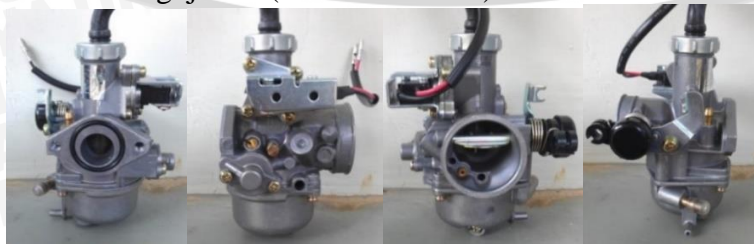
Lampiran 3. Karburator Pengujian 1 ( \varnothing venturi 18mm)
