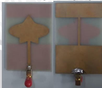
Gambar 23 Antena mikrostrip star patch with additional elliptical shape (Sumber: Fabrikasi)
