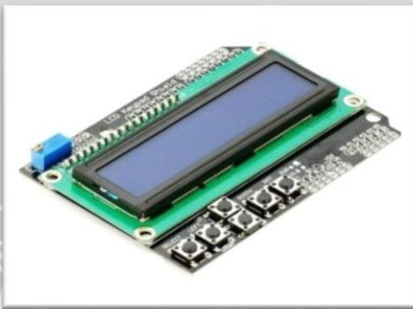
Gambar 2.13 LCD Keypad Shield (<http://www.jualarduino.com/wp-content/uploads/2013/09>)
