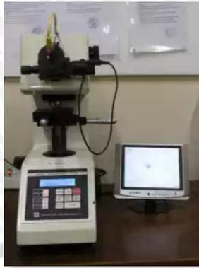
Gambar 3.3 *Digital Micro Vickers Hardness Tester*
