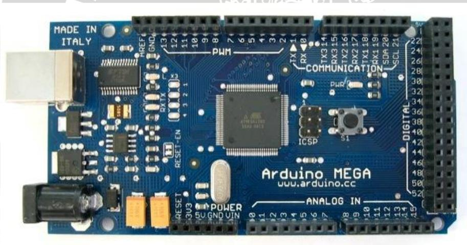
Gambar 2.7 Tampak depan Arduino Mega (<http://arduino.cc/en/Main/ArduinoBoardMega>)
