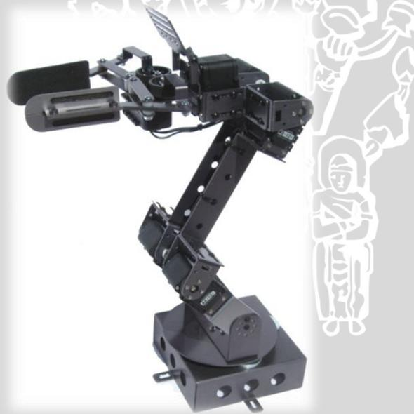
**Gambar 4.3 Smart Arm Robotic AX-12A (www.crustcrawler.com)**
