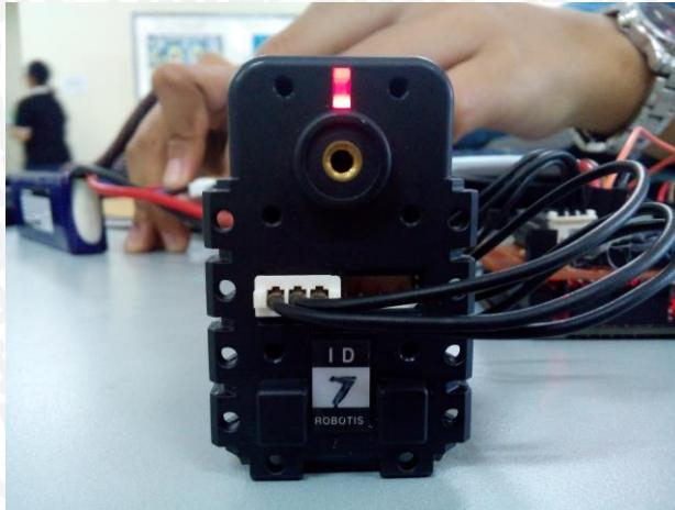
Dynamixel Digital Servo AX-12A Alarm On
