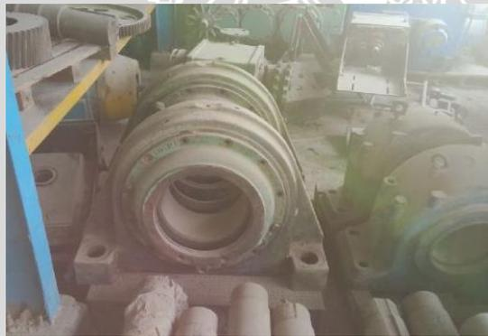
**Gambar 4.17** Seal Bearing Hammer Mill
