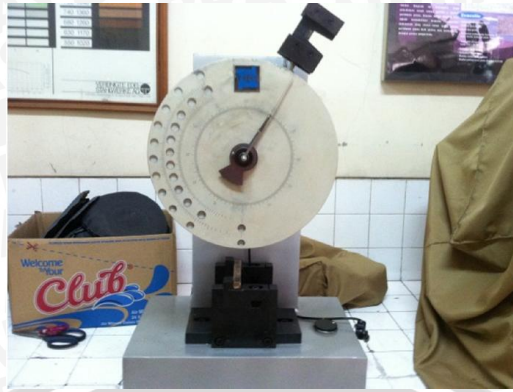
Gambar 3.1 Charpy Impact Non – Ferrous (Time Testing Machine XJJ-5)
