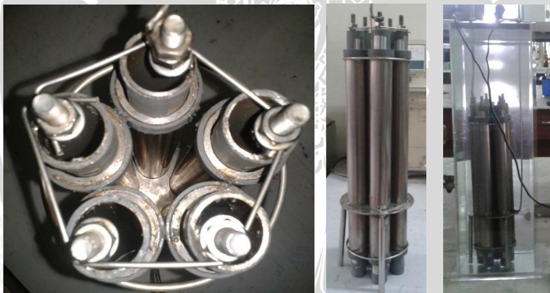
Gambar 4.3 Foto Generator Gas *Hydroxy*
