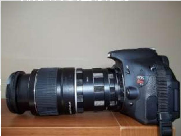
Gambar 3.12 Kamera Canon EOS 600D 18-55mm f/3.5-5.6 + Extension tube
