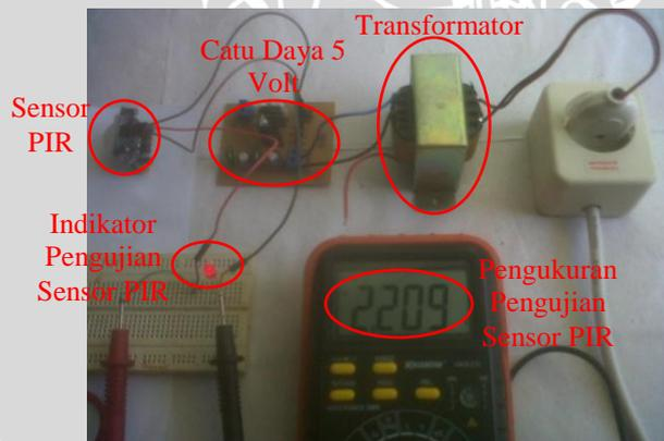
Gambar 5.1. Pengujian Sensor *Passive Infra Red*
