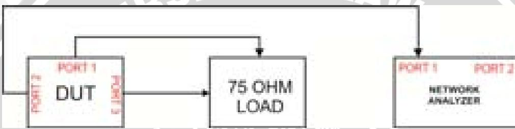
Gambar 5.2 Blok Diagram Pengukuran *Return Loss Port 2*
