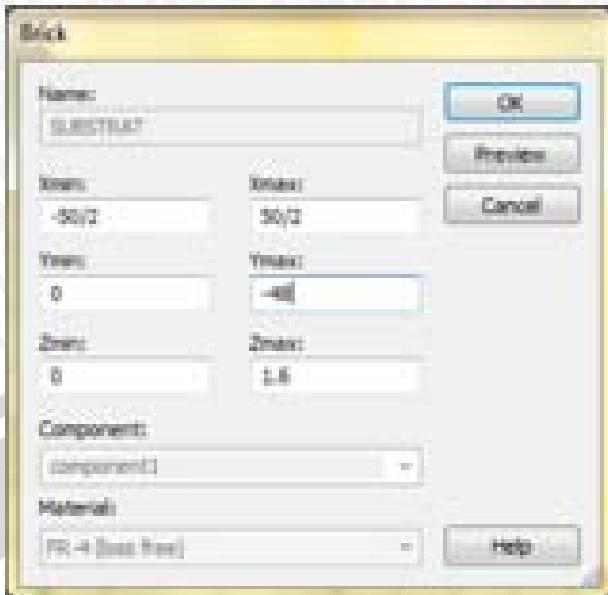
**Gambar 10.** Ukuran Balok Substrat
