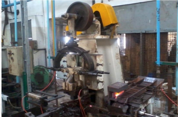
Gambar 4.3 Automatic Forging Hammer Tonase Machine Proses Produksi Kikir Sumber: PT Jaykay Files Indonesia
