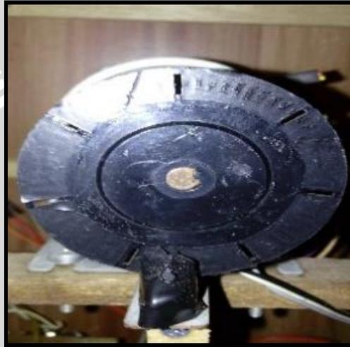
Gambar Sensor Rotary Encoder
