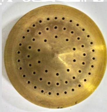
Gambar 3.11 Perforate burner material kuningan
