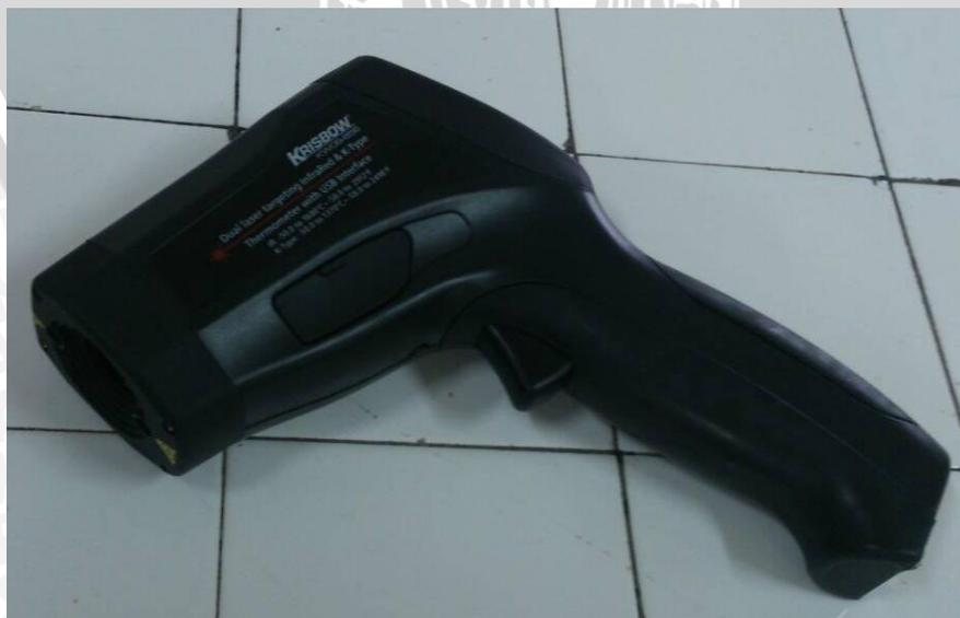
Gambar 3.5 *Infrared Thermometer Dual Laser*
