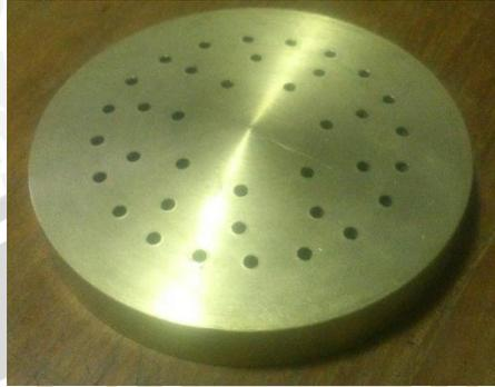
Gambar 3.12 *Perforated burner* material kuningan
