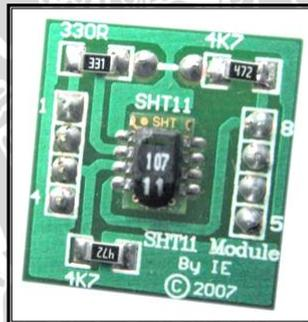
**Gambar 2.4 Sensor Suhu Dan Sensor Kelembaban SHT11**
