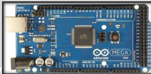
Gambar 2. 16 Tampilan Arduino Mega 2560
