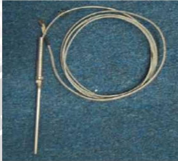
Gambar 3.5 *Thermocouple* tipe k
