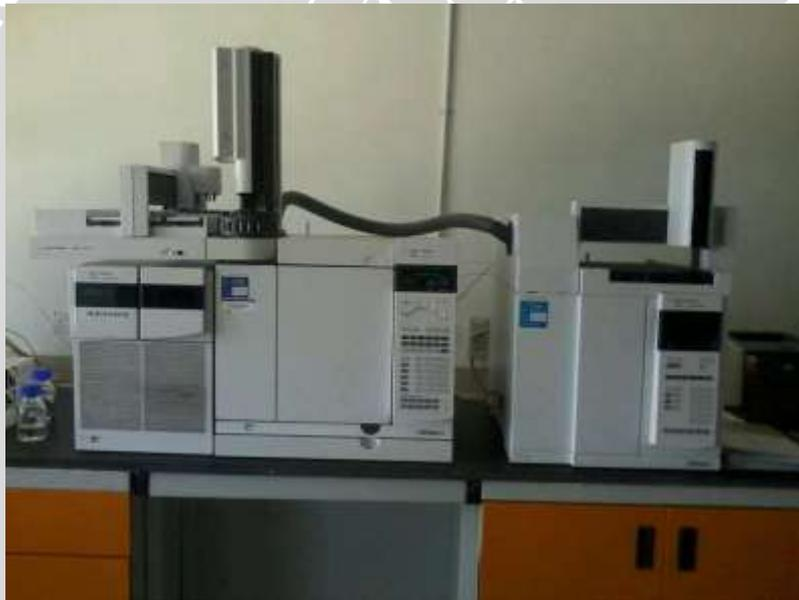
Gambar 3.10 *Gas Chromatography-Mass Spectrometry (GC-MS)*
