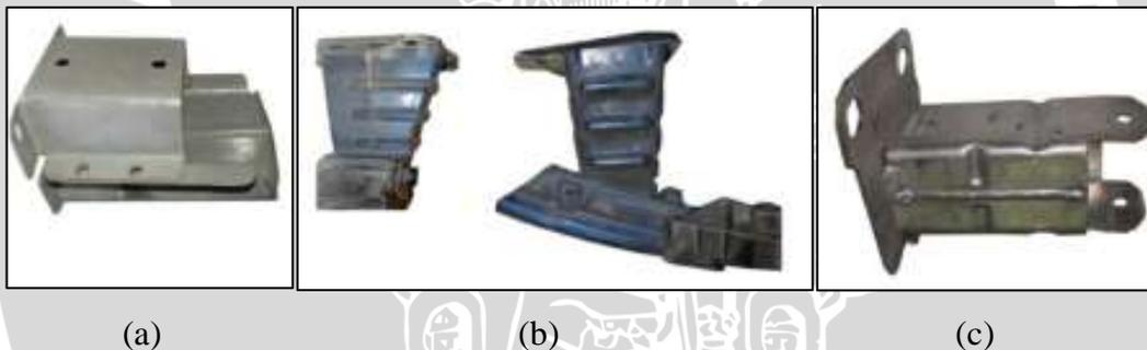
Gambar 2.8 *Crash box* (a) Honda Accord-2005 Steel, (b) Opel Astra-2006 Steel, (c) Renault Meganne/2-2008 Aluminum
