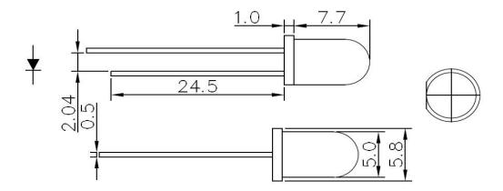
Note: Besides to the specified outside, all units in mm, a tolerance of  $\pm$  0.20mm
