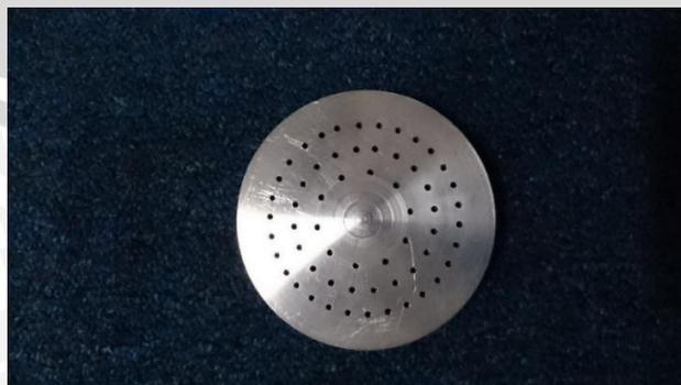
Gambar 3.5 *Perforated burner*
