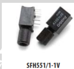
Gambar 2.4 Photo Diode SFH551/1V (Sumber: Avago, 2007)
