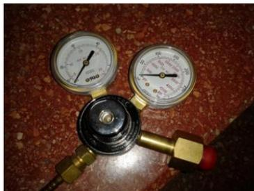
Gambar 3.8 Regulator Gas CO<sub>2</sub>
