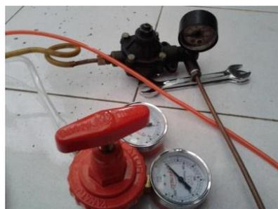
Gambar 3.7 *Regulator Gas CH<sub>4</sub>*
