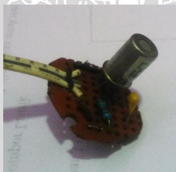
Gambar 3.10 Sensor Gas Hidrogen
